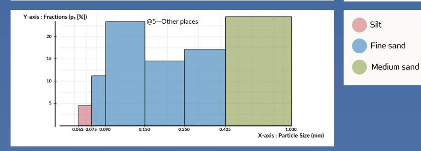
Graphs. 1-5 show the particle size distribution of soil samples collected from five different locations. Each bar indicates the percentage by weight of soil particles retained on a specific sieve size.
